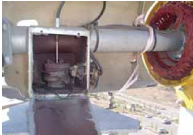
The slip ring/brush assembly on this wind generator was blasted by lightning.
