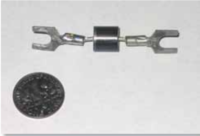
A small bypass diode from a 75-watt photovoltaic module.
