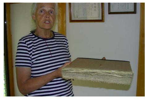
Tatami floor mats sample cross section typical of those widely used in Japan with recycling potential
